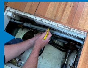
4. Mark the position for the bracket
