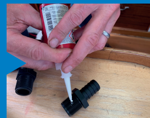
9. Using sealing compound
