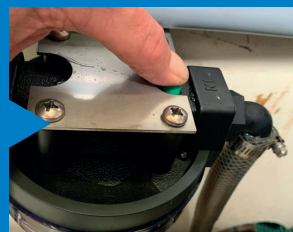
17. Bleeding air from the Wavestream
