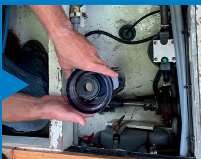
16. Placing the Wavestream into position
